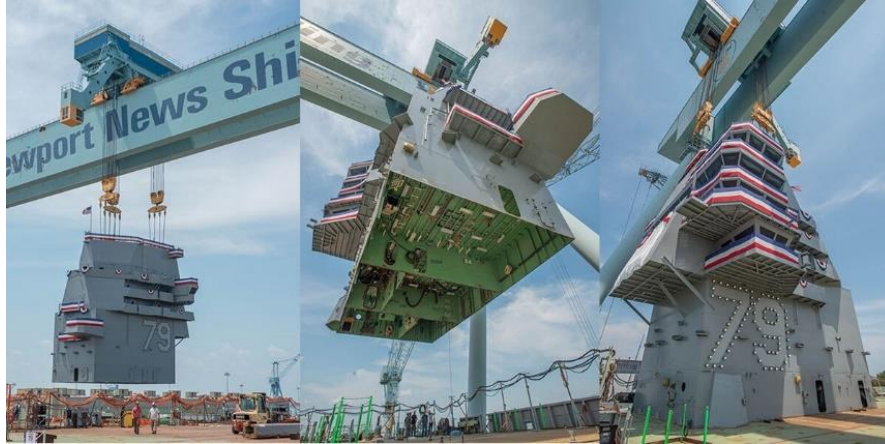
Three different views of the ship's island as it's hauled up and across the flight deck of the aircraft carrier John F. Kennedy on Wednesday at Huntington Ingalls Newport News, where the ship is being built.
